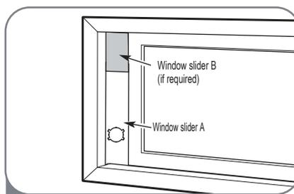
2 Insert the window slider assembly into the window opening.
