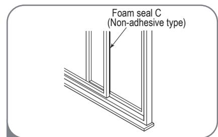
3 Cut the non-adhesive foam seal C strip to match the window height. Insert the foam seal between the glass and the window frame to prevent air and insects from getting into the room.
