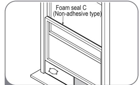
3 Cut the non-adhesive foam seal C strip to match the width of the window. Insert the seal between the glass and the window frame to prevent air and insects from getting into the room.
